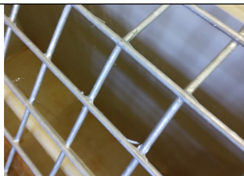
Fig. 2 : Detail of one of the galvanized meshes before test beginning.
