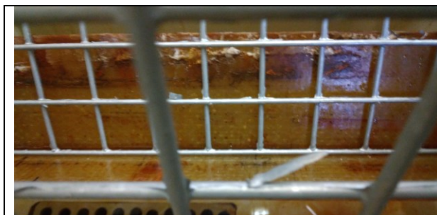
Fig. 1 : Shaped galvanized meshes showing some zinc coating burrs (before test start)
