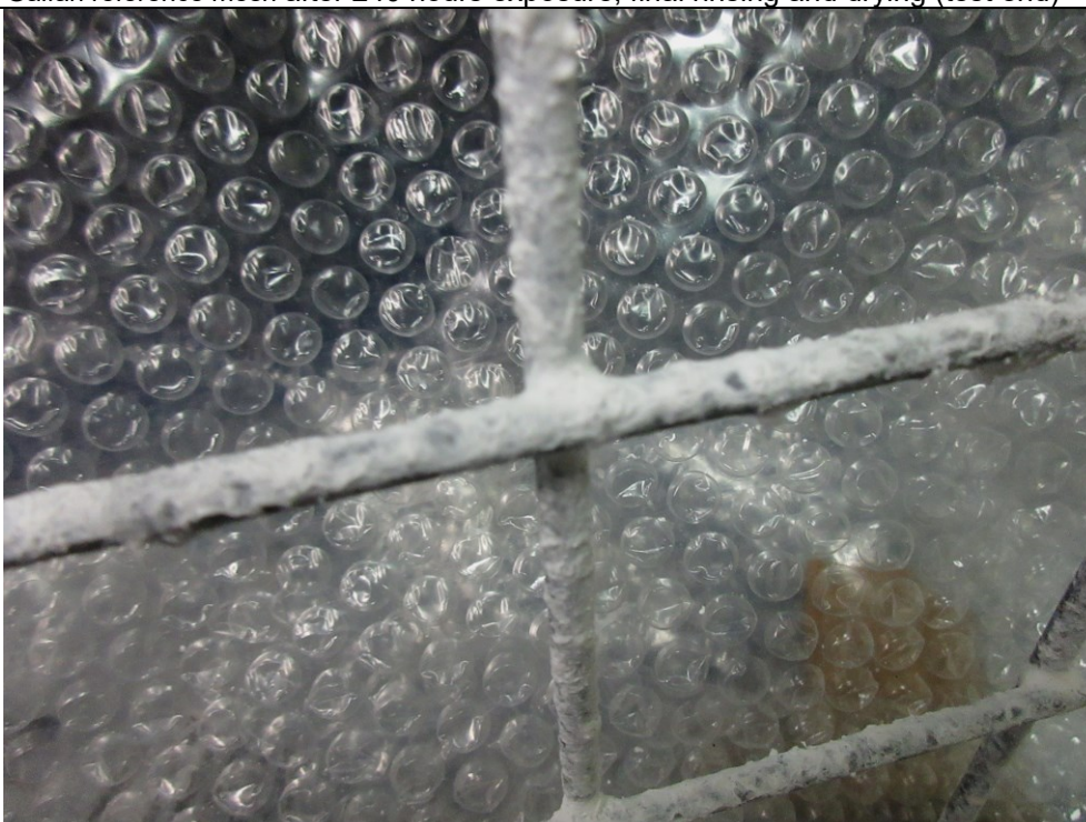
Fig. 10 : plain Galfan reference mesh – detail after 240 hours exposure, final rinsing and drying (test end)
