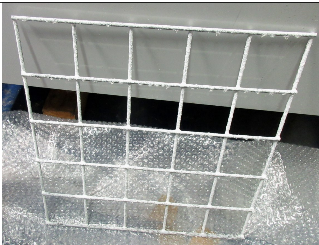
Fig. 9 : plain Galfan reference mesh after 240 hours exposure, final rinsing and drying (test end)
