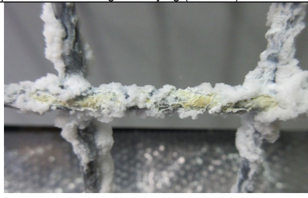
Fig. 8 : Shaped Galvanized Meshes after 240 hours exposure, final rinsing and drying (test end)
