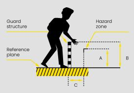
A: height of hazard zone B: height of protection guard
