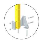
**40x40** <sup>2 M8</sup> galvanized steel mechanic plugs
