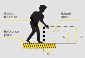
A: height of hazard zone B: height of protection guard
